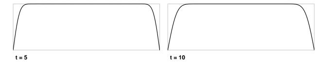
One important thing to notice is that at a mere instant after the the cooling starts, the temperature at the ends is equal to  $0^{\circ}$ . This is what 'extremely efficient' means.
