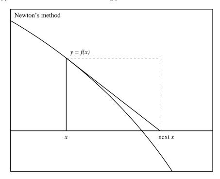
What the picture suggests is that if we have one approximation  $x_n$  to a root of f(x) = 0, then a better one can be found as the intersection of the tangent line to the graph of y = f(x), over the point  $x_n$ , with the x-axis. This intersection can be found from the definition of the derivative as slope:
