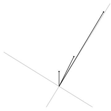
The picture suggests how to approximate the eigenvector  $v_1$ . We start with a vector  $v_0$  chosen randomly, apply A and normalize over and over again until we seem to be getting the same vector again on each iteration — that is to say, until the process has converged to the number of decimal places we are working with.
