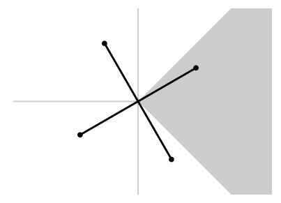
As the diagram illustrates, there will be exactly one eigenvector in the (shaded) region  $|y| \le x$ , x > 0 unless the eigenvectors lie on the lines  $y = \pm x$ . In Jacobi's method, it is this eigenvector, generally unique, which we want to pick out. We shall next see some formulas for it.
