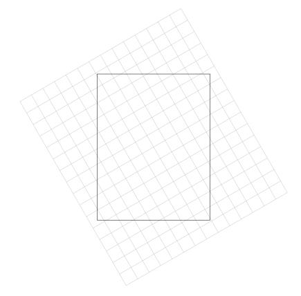
In this picture, the user coordinate system has a scale in inches, but it has been rotated by about 30°.
