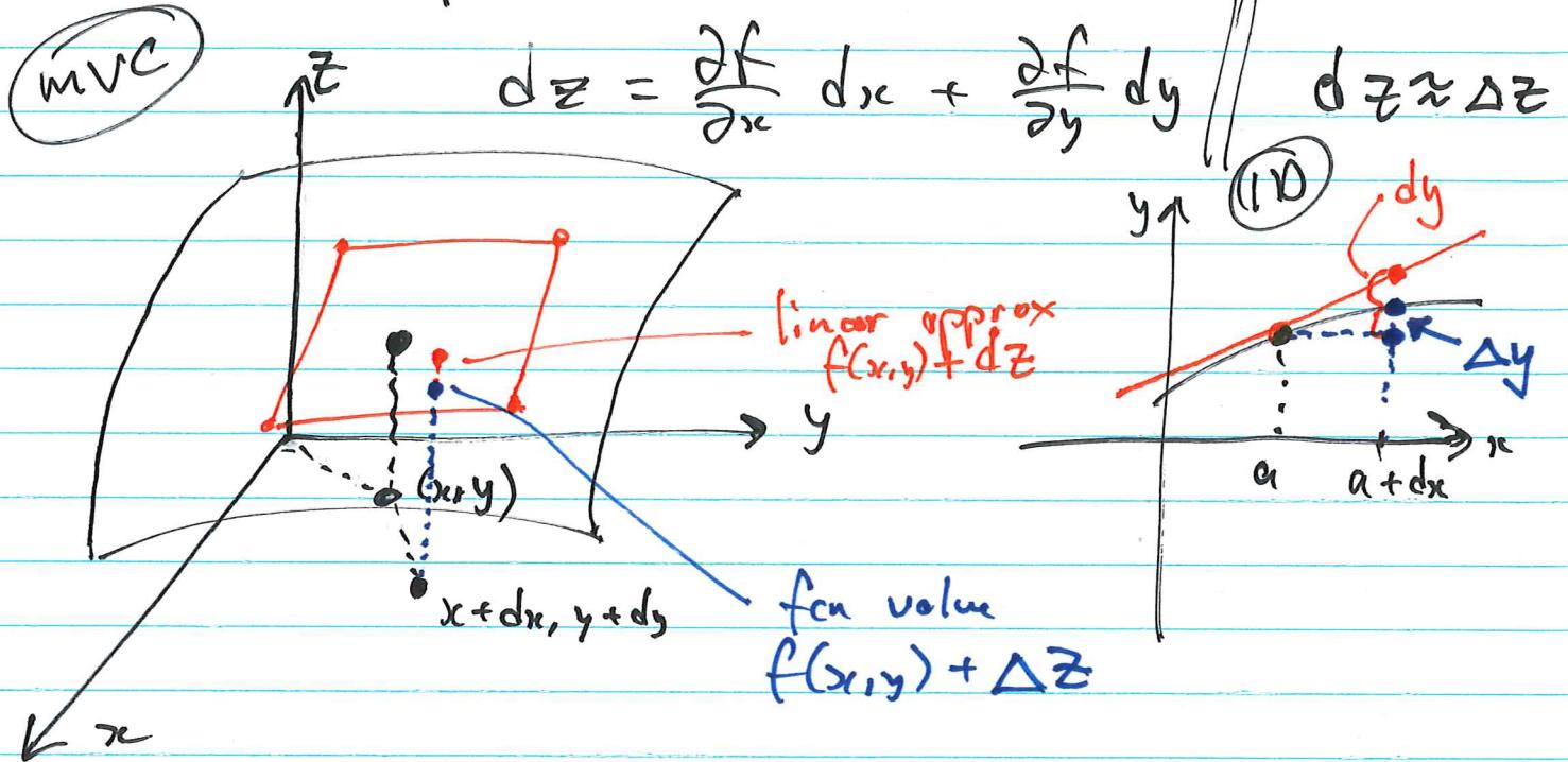
~~Ex~~ Rectangular box.  $80 \times 100 \times 50 \text{ cm}$ , measured within 1mm. Estimate the max error in the volume.
