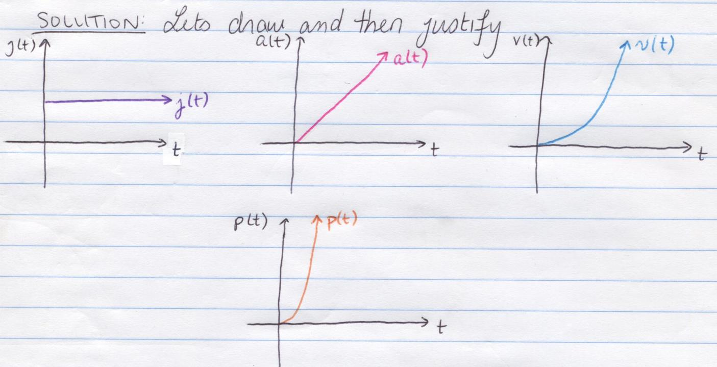
Since  $j(t)$ , i.e.  $\Delta a(t)$  is constant, we know that the rate of change of  $a(t)$  must be the same as time increases. The type of graph with this property is a line, so  $a(t)$  is linear. Similarly, since  $a(t) = \Delta v(t)$ , we know that the tangent lines of  $v(t)$  must have positive slope, and increase in slope with time.  $v(t)$  in the diagram satisfies these conditions with the slope of the tangent line at  $t=0$  being 0. Finally,  $p(t) = \Delta v(t)$  must have ....
