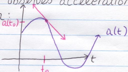
The slope of the tangent line at  $(t_0, alt_0)$  gives the instantaneous jerk, since tangent lines correspond to instantaneous rates of change.
