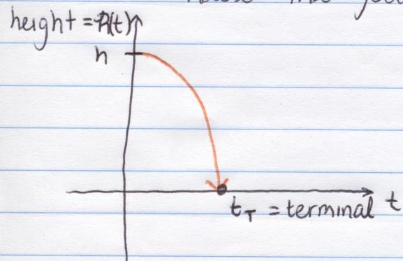
The graph is of this form since as we consider position with respect to time, at the very start of the drop, i.e.  $t=0$ , position is not changing as quickly as it does as time increases.
