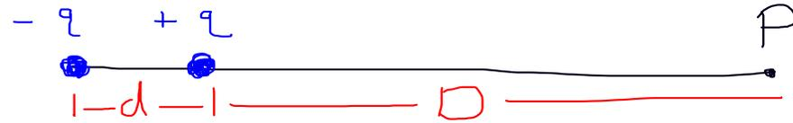
Approximate the  $E$ -field at distance  $D \gg d$  from a dipole (figure):
