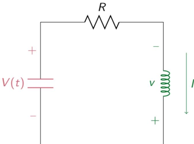
Goal: find equations for  $V(t)$  (voltage across capacitor) and  $I(t)$  (current through inductor).
