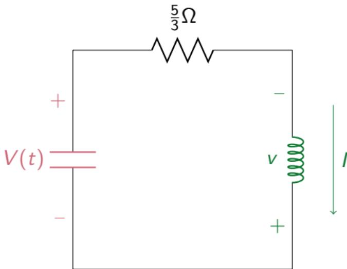
Goal: find equations for  $V(t)$  (voltage across capacitor) and  $I(t)$  (current through inductor).
