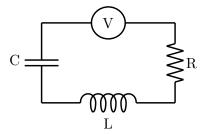
on the capacitor is Q and the current flowing in the circuit is I, the voltage across R, L and C are RI,  $L\frac{dI}{dt}$  and  $\frac{Q}{C}$  respectively. By the Kirchhoff's law that says that the voltage between any two points has to be independent of the path used to travel between the two points,
