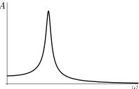
Note that there is a small range of frequencies that give a large amplitude response. This is the phenomenon of resonance. It is exploited in the design of radio and television tuning circuitry. It has also been dramatically illustrated in, for example, the collapse of the Tacoma narrows bridge.
