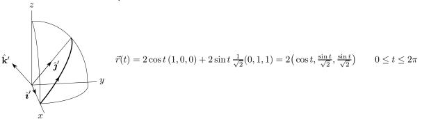
To check that this parametrization is correct, note that  $x = 2 \cos t$ ,  $y = \sqrt{2} \sin t$ ,  $z = \sqrt{2} \sin t$  satisfies both  $x^2 + y^2 + z^2 = 4$  and z = y. At t = 0,  $\vec{r}(0) = (2, 0, 0)$ . As t increases,  $z(t) = \sqrt{2}$  increases and  $\vec{r}(t)$  moves upwards towards  $\vec{r}(\frac{\pi}{2}) = (0, \sqrt{2}, \sqrt{2})$ . This is the desired counterclockwise direction. Now that we have a parametrization, we can set up the integral.
