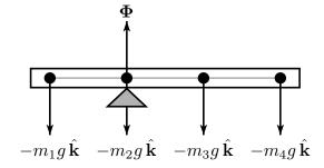
external force is  $\mathbf{F} = \mathbf{\Phi} - \sum_{i=1}^{n} m_i g \hat{\mathbf{k}} = \mathbf{\Phi} - M g \hat{\mathbf{k}}$ . If the seesaw is to remain stationary, this must be zero so that  $\mathbf{\Phi} = M g \hat{\mathbf{k}}$ . The total torque (about the origin) is
