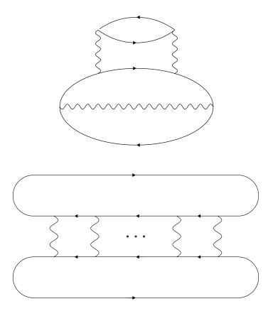
The directed and wavy bonds are called particle and interaction lines respectively. Joining a pair of legs produces one particle line.
