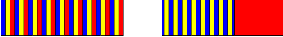
Figure 2: Left plot: the ABC\dots ABC lamellar morphological phase found in triblock copolymers. Right plot: the ABAB\dots ABAC phase found in homopolymer/diblock copolymer blends.
