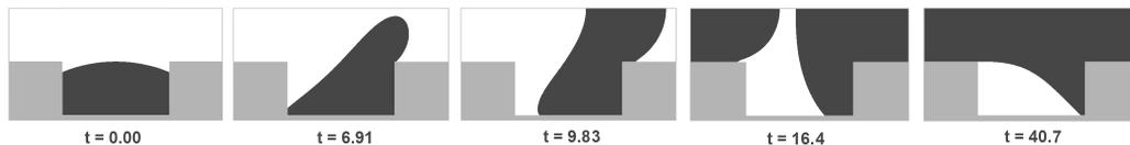
Figure 6: Development of the liquid flow regime with  $F = 0.75$  and  $S = 0.38$ . Because of the axisymmetry of the geometry, as the liquid moves from the chamber into the pore throat, its projected area on the meridian plane being plotted increases even though its volume is conserved.
