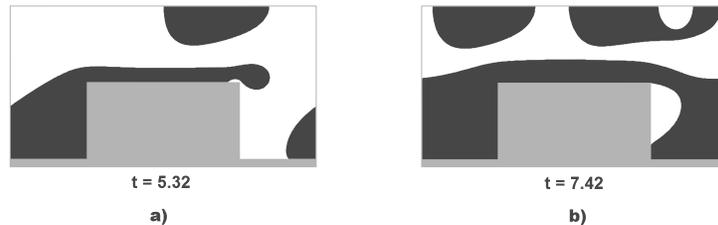
Figure 9: Variants of the annular flow regime: (a) droplet flow at  $F = 3$  and  $S = 0.31$ ; (b) annular-droplet flow at  $F = 3$  and  $S = 0.75$ . Both are time-periodic configurations, and the liquid film on the ridge in (a) has stopped moving downstream.
