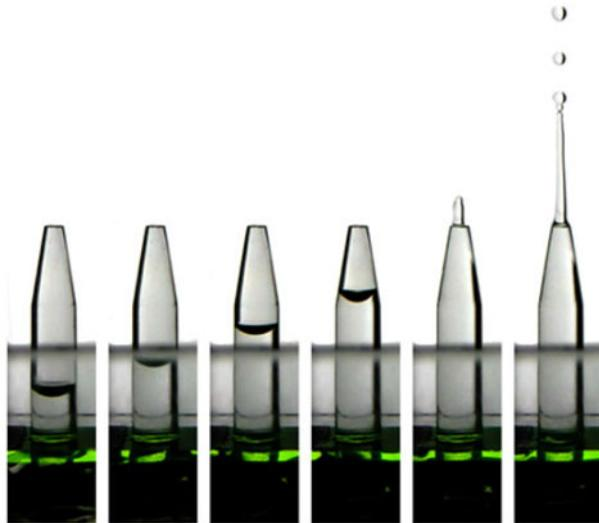
FIGURE 1. (Colour online) A sequence of snapshots showing spontaneous capillary rise and auto-ejection of droplets in the experiment of Wollman & Weislogel (2013) under microgravity. The inner diameter of the glass tube is 9.2 mm in the straight section, and the liquid is PDMS of viscosity 0.65 cs. The drop volume is roughly 20  $\mu\text{l}$ . The photos are taken 0.1 s apart. Adapted from Wollman & Weislogel (2013) with permission, ©Springer.
