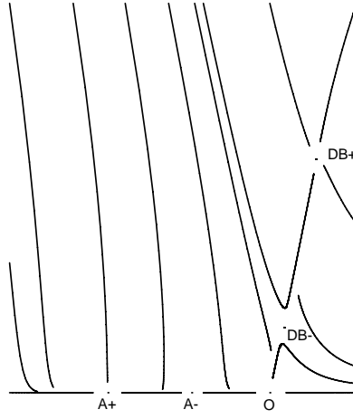
Figure 6: Phase portrait of the bifurcation equations for the Brusselator model when \sigma_2 < \sigma_{max} < 0 . The patternless solution O , annular pattern solution A+ and dichotomous branching pattern solutions DB+ are stable. The annular pattern solution A- and dichotomous branching pattern solutions DB- are unstable.
