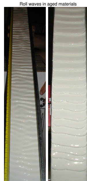
FIG. 3: Roll waves on fluid layers of aged material. The second panel shows an experiment in which the inclination was steeper than that shown in the first panel.
