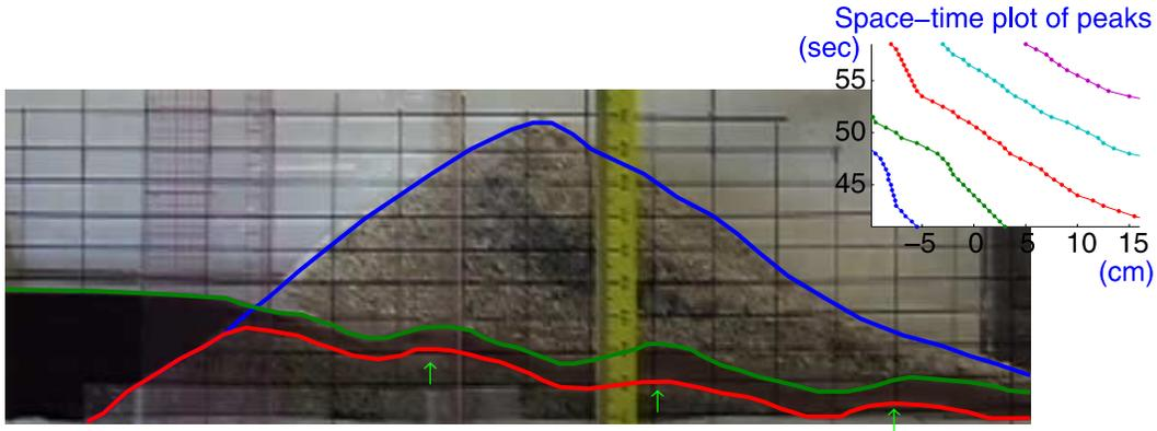
**Figure 5.** A photograph showing bed forms during a dam breach. Lines highlight the water surface, bed elevation and the relic of the original dam in the background. The inset shows a plot of the spatial positions of the maxima in the bed as functions of time.
