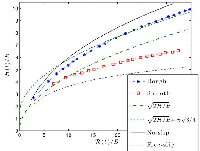
**Fig. 14.** Maximum radius  $\mathcal{R}(t)/B = \rho g \hat{R}/\tau_Y$  versus depth  $\mathcal{H}(t)/B = \rho g \hat{H}/\tau_Y$  for experimental extrusions with a pump rate of 31.5 ml/min over the rough (stars) and smooth (squares) plexiglass. Also plotted are the leading-order and improved asymptotic predictions, and Herschel–Bulkley simulations matching the physical parameters of the experiment with either no slip or free slip boundary conditions.
