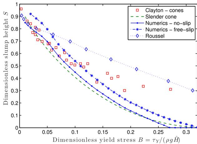
**Fig. 16.** Slump heights for Bingham dambreaks with an initially conical shape corresponding to the ASTM standard, computed using a no slip (solid line with points) or free slip (dashed-dotted line with stars) condition on the underlying plane. Squares show experimental data from [4]. The dashed line shows the prediction for a slender conical column in Appendix D. The diamonds show the results of numerical computations of [9].
