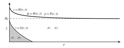
FIGURE 1. A schematic showing the depth h(r, t) of the injected fluid and the uplift H(r, t) of the overburden, associated with an injected flux Q at r = 0. The porosity and fluid pressure at z = H are given by  $\phi = \Phi(r, t)$  and p = P(r, t), respectively. Before any fluid is injected,  $H = H_0$ ,  $\Phi = \Phi_0$  and  $P = \mathcal{P}$ , where  $\mathcal{P}$  is the overburden pressure.
