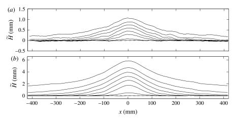
FIGURE 7. Experimental measurements of the height  $\widetilde{H}$  of the deviation of the upper surface, in mm, at times t=2, 4, 8, 16, 32, 64, 128 and 256 s. (a) Injection rate  $Q=25~{\rm cm}^3~{\rm min}^{-1}$ . (b)  $Q=200~{\rm cm}^3~{\rm min}^{-1}$ . The coordinate x measures the radial distance from the point of injection, such that r=|x|.
