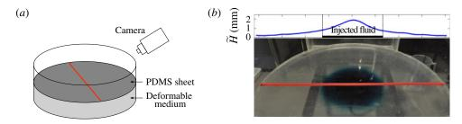
FIGURE 6. (Colour online) (a) A schematic of the experimental set-up. (b) An image from an experiment in which the injected water was dyed blue to distinguish it from the clear ambient water. The profile above shows the uplift of the upper surface, as measured by the deflection of the line on the PDMS sheet, and demonstrates that the uplift travels ahead of the blue fluid. The flux was Q = 100 cm<sup>3</sup> min<sup>-1</sup> and the image was taken roughly 2 min after the start of injection.
