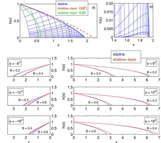
FIG. 3: TOP: (a) Slipline field and surface profiles for  $B = 0.8$  and  $\phi = 0$ , (b) detail near the slump edge.
