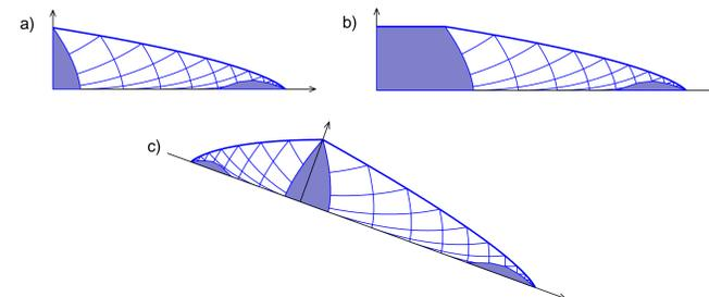
FIG. 2: The slipline field can be joined to (a) a stagnant wedge abutting a back wall, (b) an upstream layer of unyielded fluid, or (c) an unyielded core separating deposits slumped in either direction.
