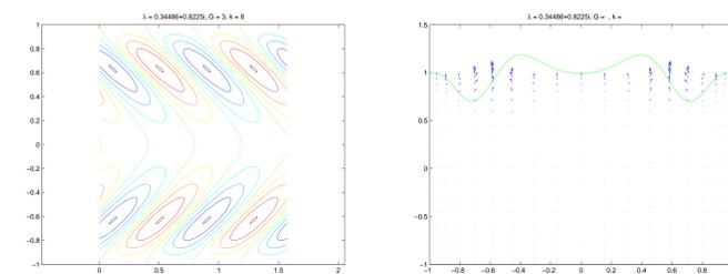
FIGURE 4: (a) The out-of-plane perturbation profiles as functions of  $x$  and  $y$  for the most unstable mode. (b) Cross-sections of the out-of-plane displacement (exaggerated) and cross-sectional velocity fields. The parameters are  $G = 3$ ,  $k = 8$ ,  $\delta = 0.1$  and  $\nu = 0.3$ .
