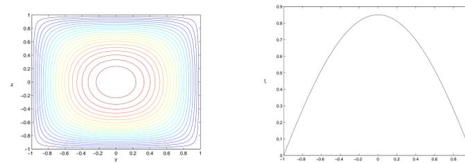
FIGURE 2: The base state down-slope (a) fluid velocity contours and (b) plate displacement for  $\nu = 0.3$  and  $G = 1$ .
