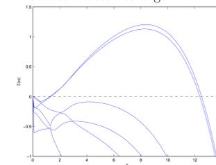
FIGURE 3: The growth rate,  $\Im(\omega)$ , as a function of wavenumber for the most unstable modes for  $G = 3$ ,  $\delta = 0.1$  and  $\nu = 0.3$ .
