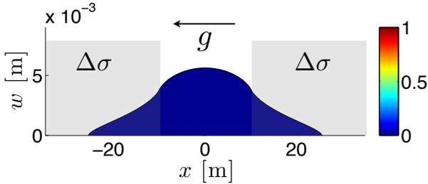
Figure 2: Variation of the width of the fracture versus the  $x$  coordinate for a KGD fracture with stress barriers at  $t = t_{\text{end}}$ . Colour filling indicates proppant concentration.
