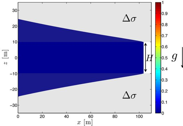
Figure 5: Fracture footprint for the P3D fracture with stress barriers at  $t = t_{\text{end}}$ . Colour filling indicates proppant concentration.
