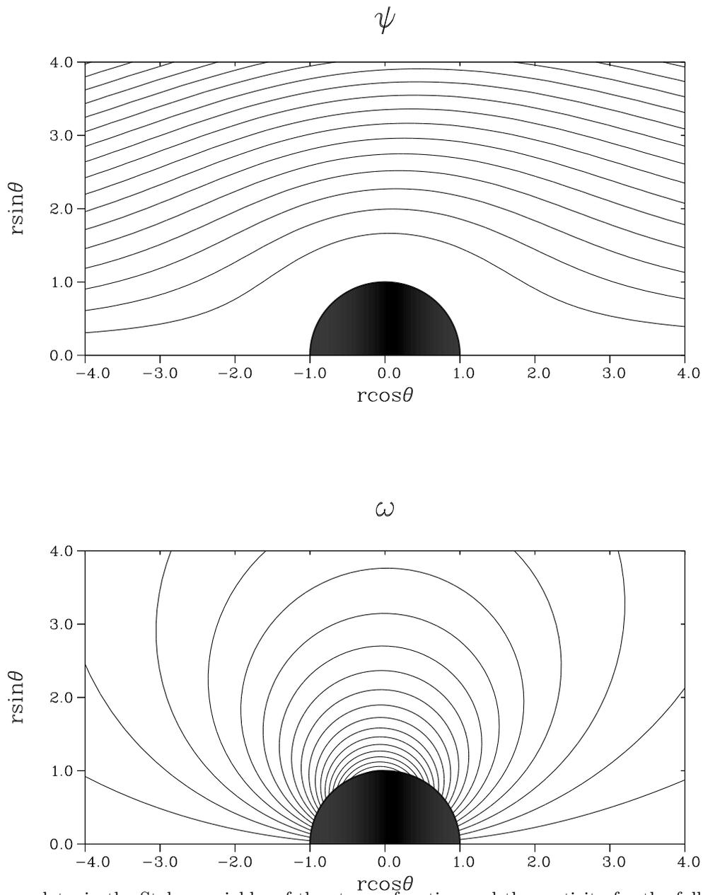
Fig. 7: Contour plots, in the Stokes variable, of the stream function and the vorticity for the full flow over a circular cylinder computed from (4.13) with  $\epsilon = 0.085$ . Notice that the full flow field has a very slight upstream/downstream asymmetry.
