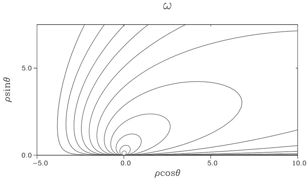
Fig. 8: Contour plots, in the Oseen variable, of the stream function and the vorticity computed from the hybrid problem (4.10) with  $\kappa = 0.25$  ( $\epsilon \approx 0.085$ ).
