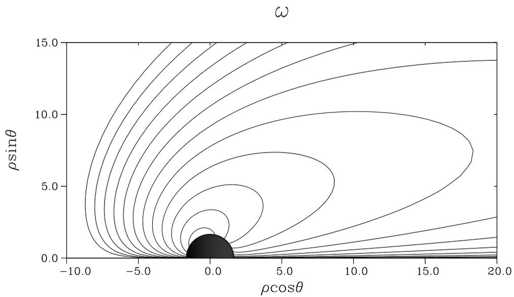
Fig. 11: Contour plots, in the Oseen variable, of the stream function and the vorticity computed from the full problem (4.13) with  $\epsilon = 1.65$ .
