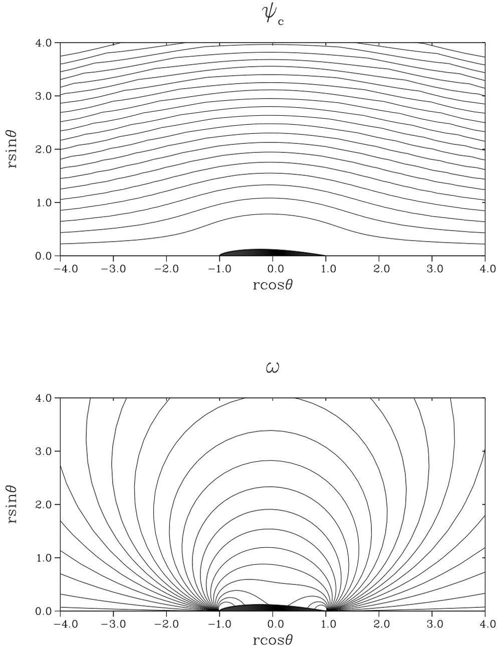
Fig. 5: Contour plots of the stream function and the vorticity, computed from (4.5), for Stokes flow around the Karman-Trefftz airfoil (4.7) with  $\kappa = 1.91$  and  $c = 0.954$ .
