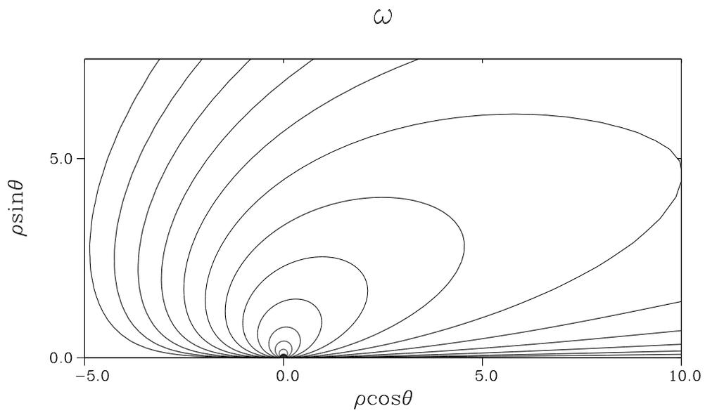
Fig. 9: Contour plots, in the Oseen variable, of the stream function and the vorticity computed from the full problem (4.13) with  $\epsilon = 0.085$ .
