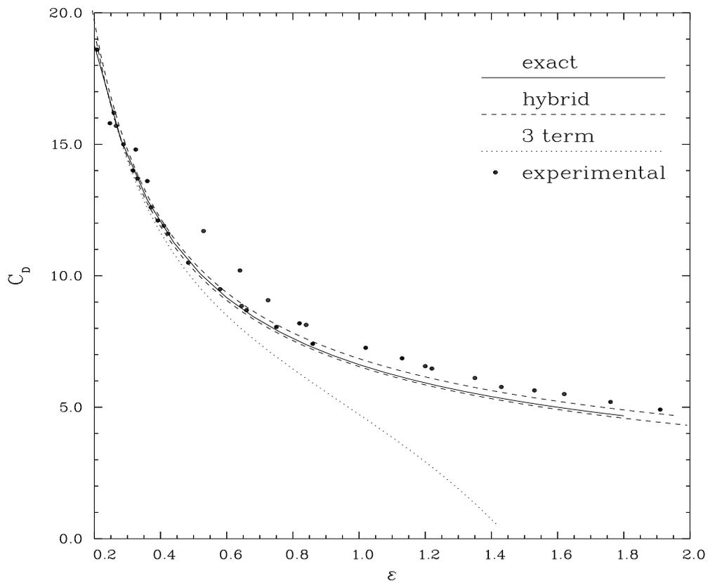
Fig. 6: For a circular cylinder, the hybrid results for  $C_D$  versus the Reynolds number  $\epsilon$  are compared with experimental results, with the three-term expansion (3.10b), and with the full numerical results. The top hybrid curve corresponds to  $A_{max}^*$  and the bottom curve corresponds to  $A_{min}^*$ .
