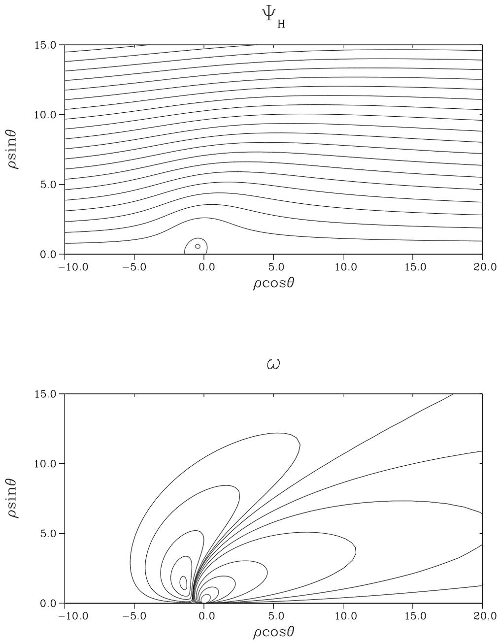
Fig. 10: Contour plots, in the Oseen variable, of the stream function and the vorticity computed from the hybrid problem (4.10) with  $\kappa = 0.65$  ( $\epsilon \approx 1.65$ ).
