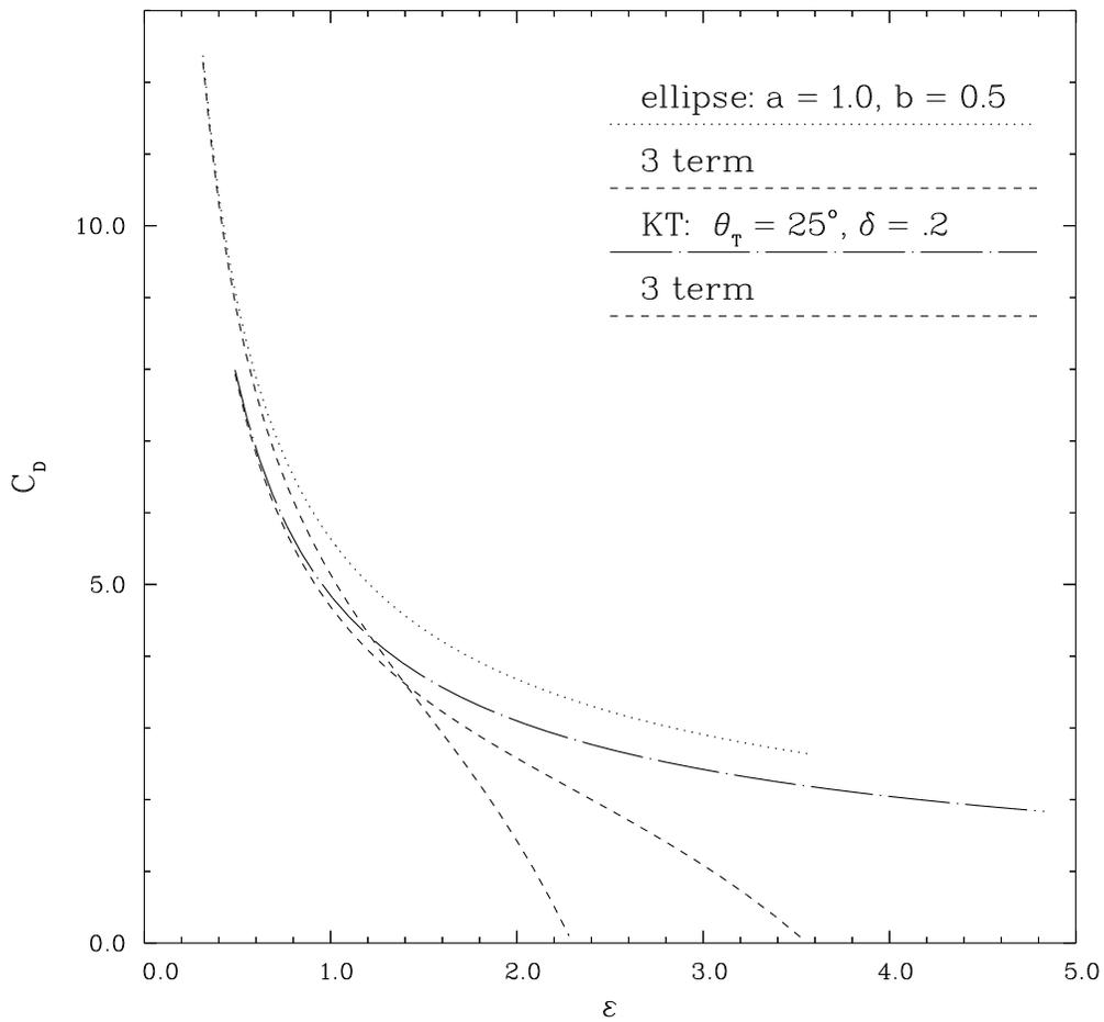
Fig. 13: The hybrid drag coefficient is compared with the three-term result (3.10b) for a cylindrical body with either an elliptical or a Karman-Trefftz airfoil cross-section.
