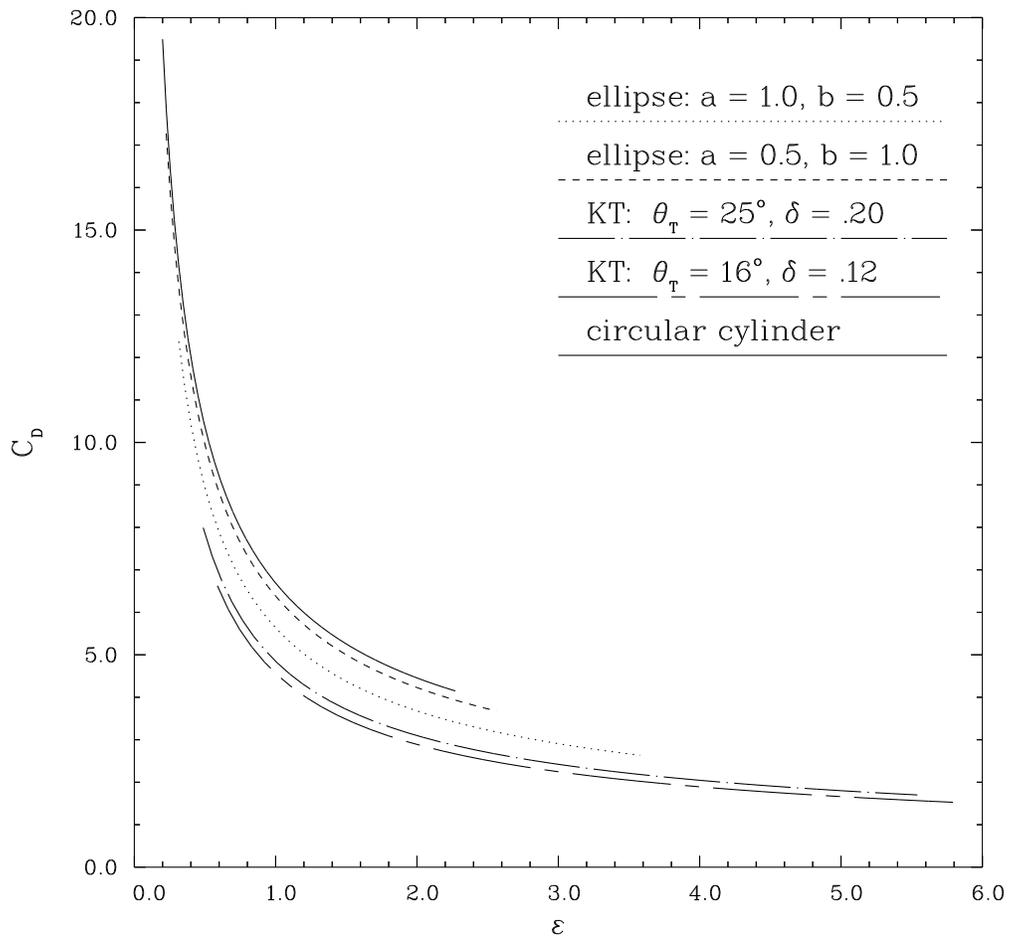
Fig. 12: Plots of the hybrid drag coefficient for cylinders of various cross-sectional shapes.
