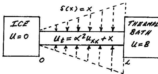
FIGURE 1. Bar subject to a time-independent heat source distributed along its length with inhomogeneous Dirichlet BC
