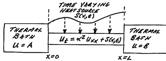
FIGURE 2. Bar subject to a time dependent heat source distributed along its length with inhomogeneous Dirichlet BC
