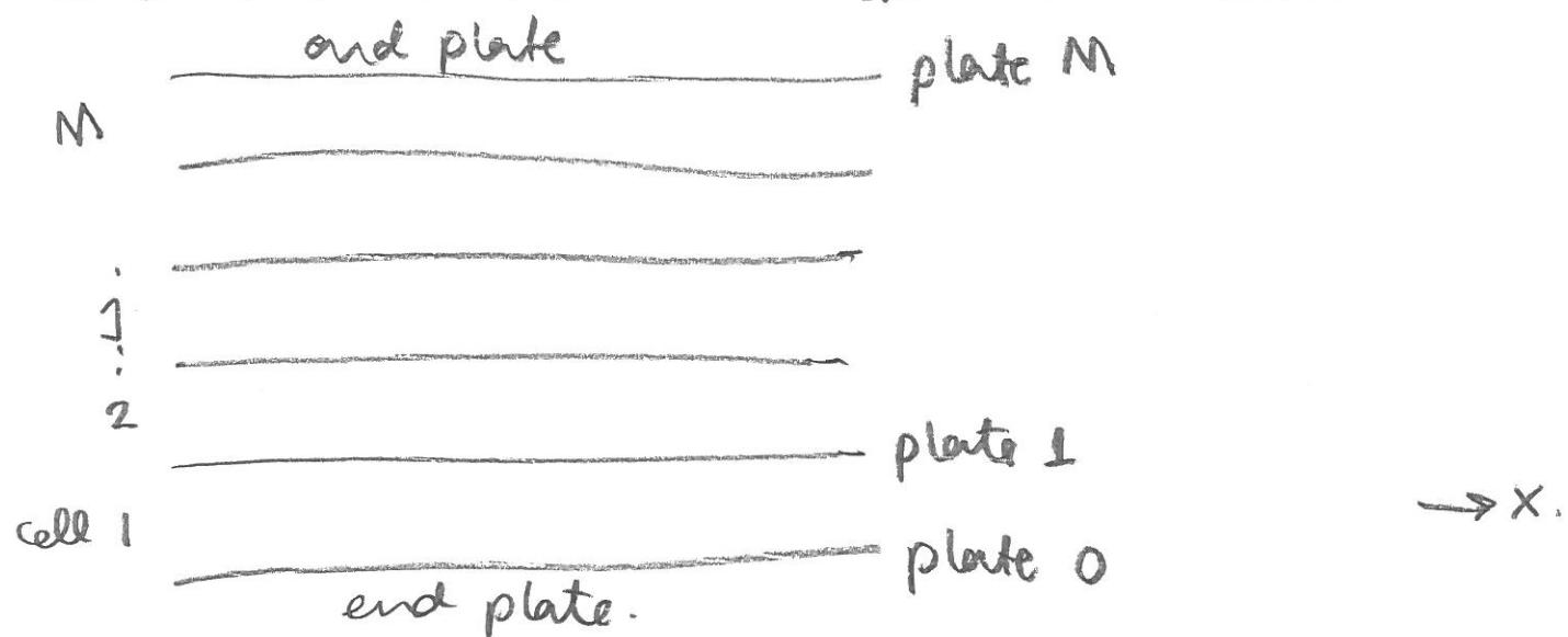
$M$  cells, assume that each cell is at the same pressure ( $P_{tot}$ ) and temperature  $T$ . However, we will allow the inlet flow rates  $\{S_m\}$ ,  $m = 1, \dots, M$  to vary.
